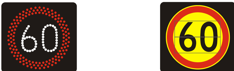
Figure 2. Schematic representation of the LED or fibre-optic sign (left) and the electromechanical sign with black background square (right).
