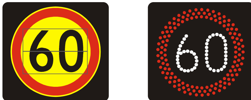
Figure 1. Schematic representation of (left) the electromechanical sign and (right) the fibre-optic sign.
