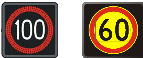
Figure 2. Schematic pictures of a LED/fibre optic and an electromechanical speed limit sign.
